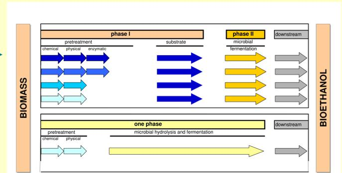
Schematic representation of bioethanol production: double and single step.
